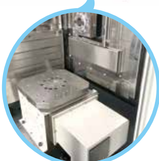
獨立工作台面能穩定長期加工的定位精度 The independent table make the positioning of the long-term processing more precise, stable
