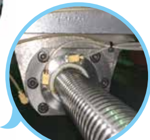
滾珠螺桿螺帽冷卻裝置 Nut screw coolant device in the ball-screw
