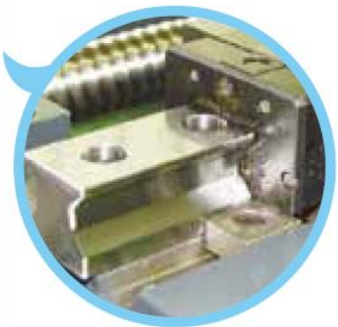
45mm PMI (SP級)滾柱型線性滑軌及荷重型滑塊
